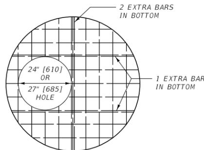
TYPE 3 MANHOLE ROOF SLAB
