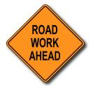
The purpose of this guidance is to provide MDT field crews and Transportation Management Plan (TMP) teams with help in the use of the W20-1, Road Work Ahead, advanced warning sign.
