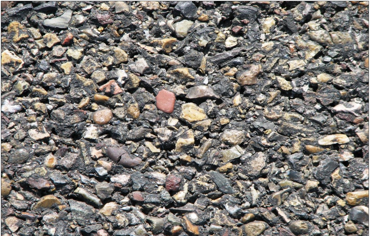
↑ ↓ Representative Images of PMS surface texture. No abnormal surface deformation noticed. No apparent bleeding or raveling is perceptible throughout the project. Polishing of aggregate minimum.
