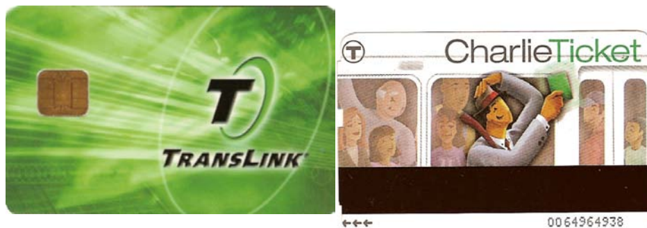
Figure 2: Magnetic Stripe and Smart Cards
