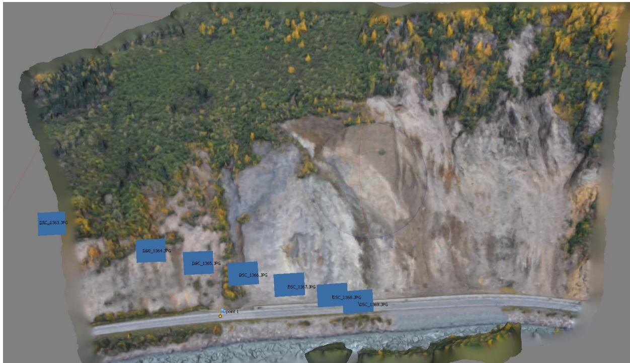
Figure 16: Parks Highway PhotoScan surface model. Blue squares indicate helicopter positions. This low density surface consists of 1.6 million points and 323,000 TIN faces.
