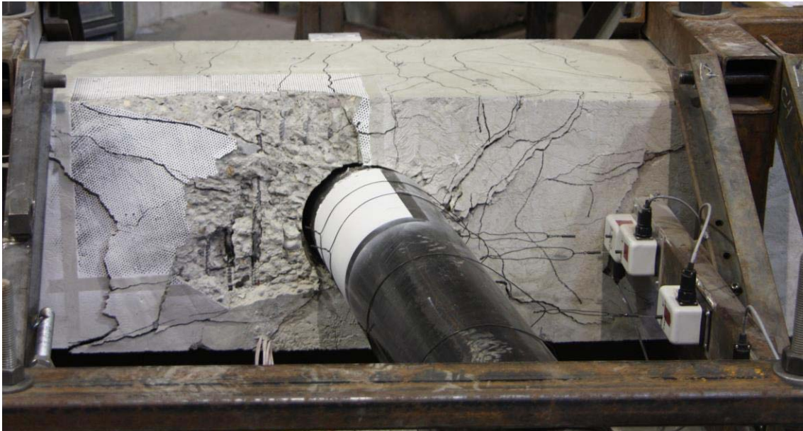
Figure 38: VT2 Failure at maximum deflection on return pull
