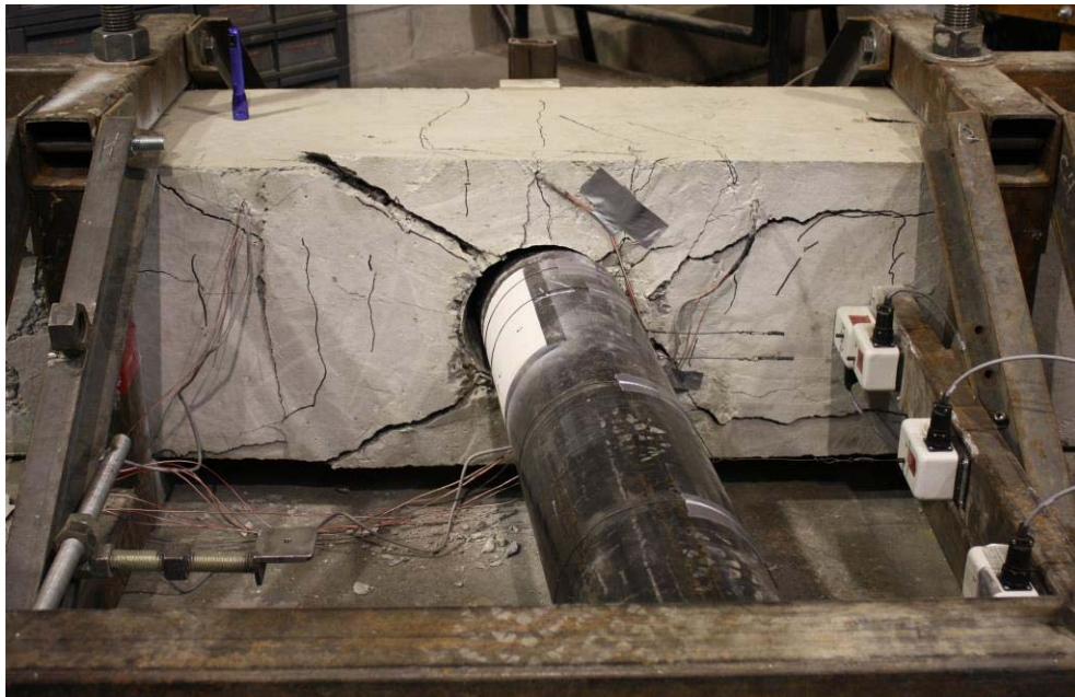
Figure 46: VT3 Failure at maximum deflection on initial pull
