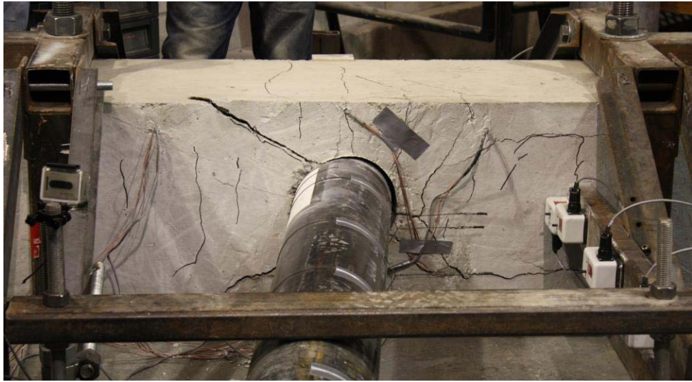
Figure 45: VT3 Failure at maximum deflection on initial push
