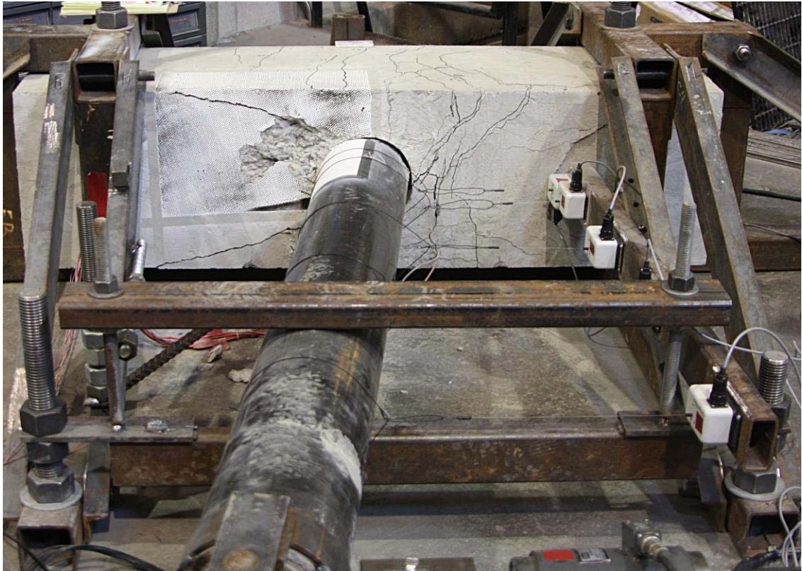
Figure 37: VT2 Failure at maximum deflection on initial push
