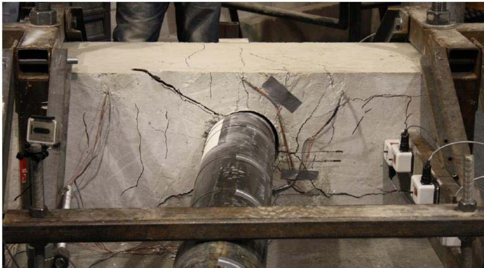
Figure 20. Typical cap at failure
