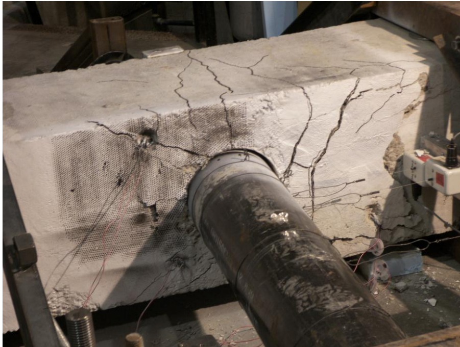
Figure 41: VT2.5 Failure at maximum positive deflection
