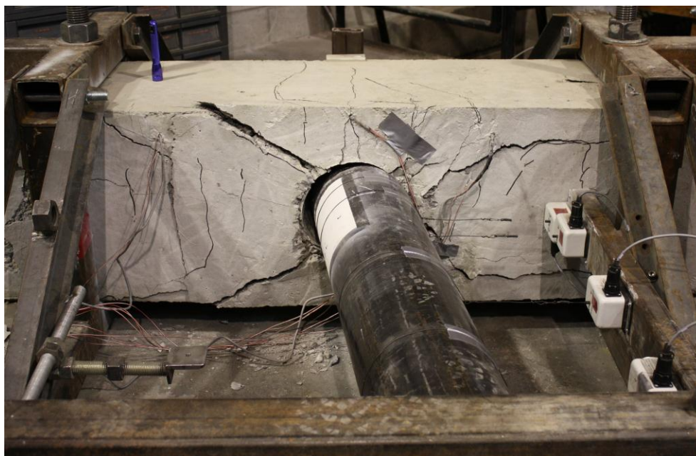
Figure 46: VT3 Failure at maximum deflection on initial pull
