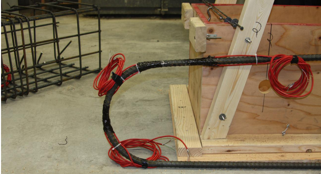
Figure 29: Typical strain gage placement on U-bar
