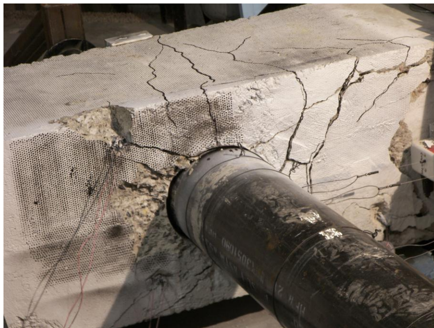
Figure 42: VT2.5 Failure at maximum negative deflection
