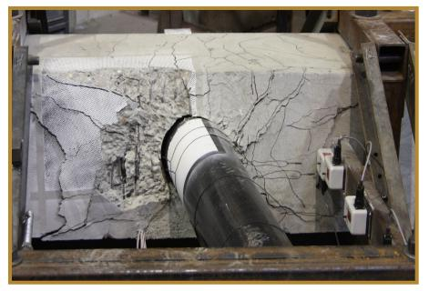
Figure 4 - Typical Pile Cap Near the Completion of Testing
