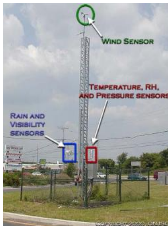
Figure 16. A RWIS sensor station (Boon and Cluett 2002)
