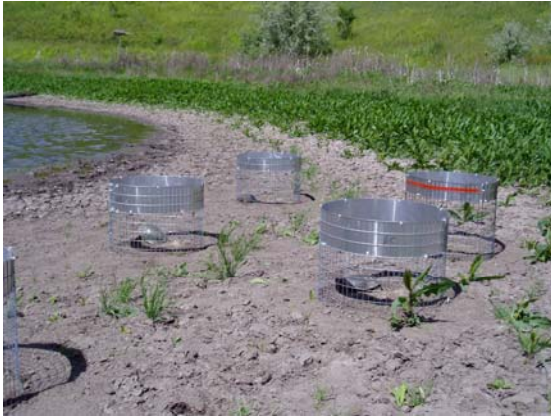
Figure B-1. Wire enclosures with aluminum flashing used to test turtle's climbing ability.
