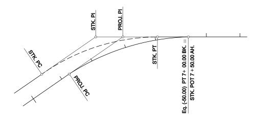
Note: If back station > ahead station, equation is (+). If back station < ahead station, equation is (-).
