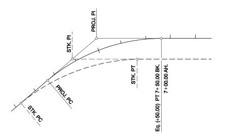
EQUATION WHERE DESIGN LINE BECOMES PARALLEL WITH STAKED LINE Figure 25.6H
