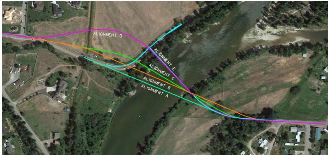
Figure 3-1. Roadway Alignment Options
