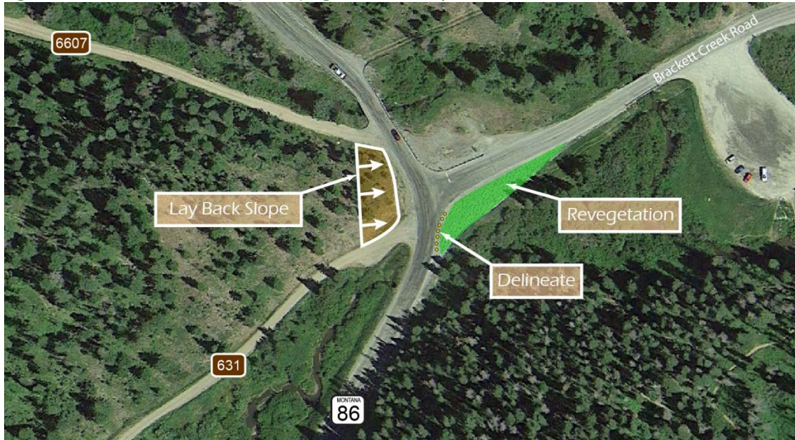
Figure 10 Brackett Creek (RP 18.8) Sight Distance Improvements
