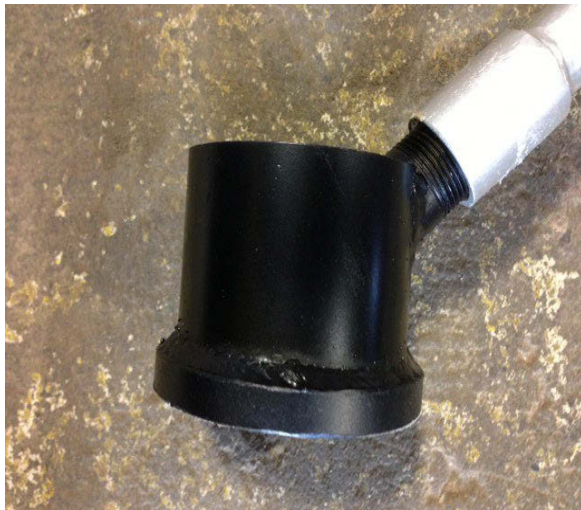
Figure 4: Crack sealing cup
