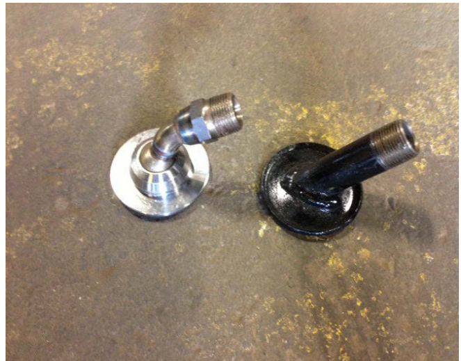
Figure 5: Crack sealing puck
