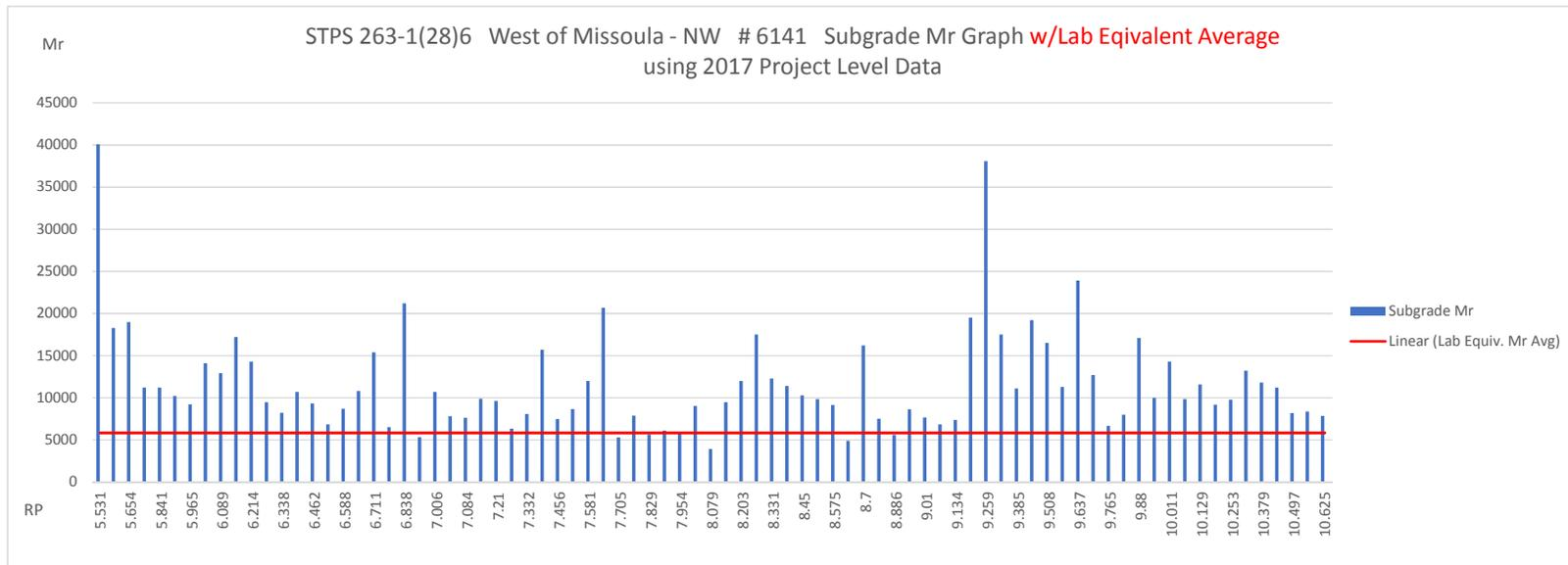
Figure 3A-1. Backcalculated Subgrade Modulus Values obtained from MDT Surfacing Section.
