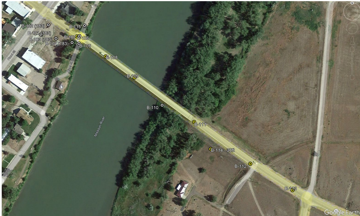
Figure 1-2. Proposed Geotechnical Boring Locations
