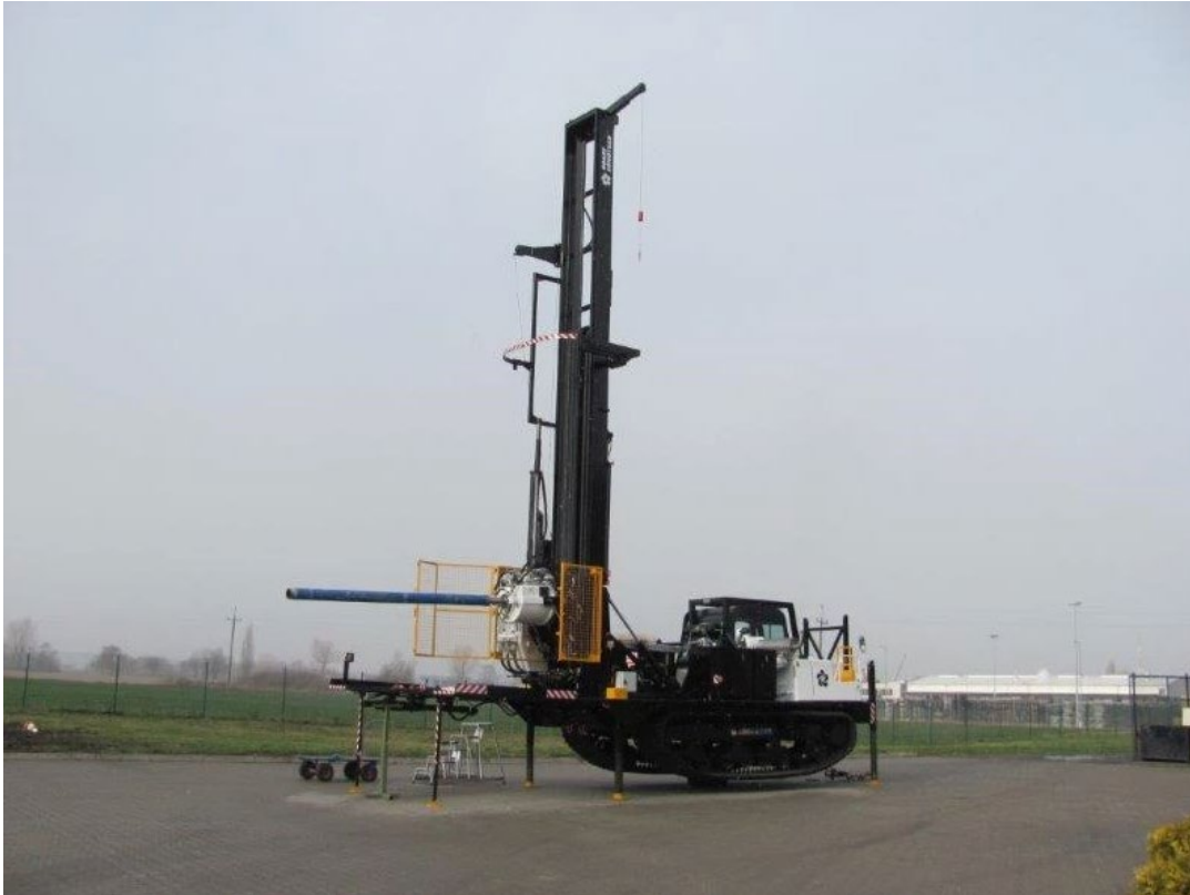
Figure 1-3. Typical Sonic Drill Rig
