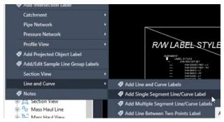
Click on each end of the line to place the distance and bearing label. Leave this label on layer VL-PLSS-TIEL-NPLT in the file for checking.
