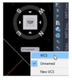
To rotate the cross hairs back, in the Command Line type PLAN, select World.
