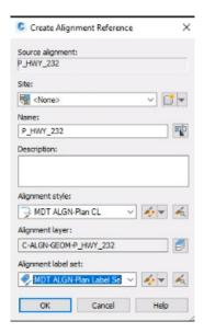
Before placing proposed right-of-way the alignment will need to be promoted into the ROMAP file. Promoting the alignment makes it an independent object that is no longer automatically updated if the original source is edited. After receiving notification that the road design alignment is final, check to see if the promoted right-of-way baseline needs to be updated.
