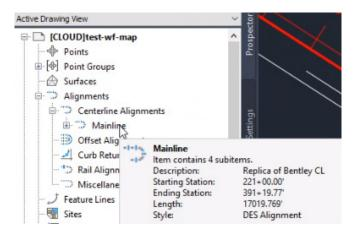
In the Create Alignment Reference box that appears change the Name to RWBL. The Alignment layer will update to include RWBL. For additional right of way baselines use a logical name such as RWBL\_JohnsonLane.
