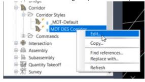
Turn off Region Boundaries and Assembly Insertion Stations. Select Make a local copy of the style. The constructions limits should be displayed properly.
