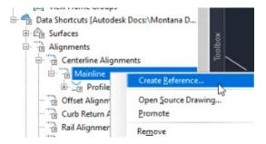
This data shortcut will have the name and layer assigned to it by road design. It's important that this data shortcut remain on its own layer so it does not get mixed up with the r/w baseline.
