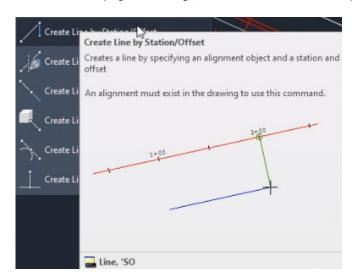
Typing LINE, keyin L, hit enter, type 'SO will bring up the Create Line by Station/Offset tool. This tool is also located on the Transparent Commands toolbar.
