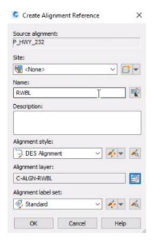
If the Create Alignment Reference box does not appear when the alignment is promoted, use the steps below to change the alignment name and layer. Right click on the promoted alignment, select Properties, change the name to RWBL. Go to Layer Properties Manager, select the alignment and Rename Layer to C-ALGN-RWBL.
