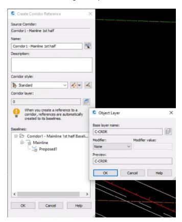
Set the Corridor style to MDT DES Corridor to display the construction limits. Select OK.
