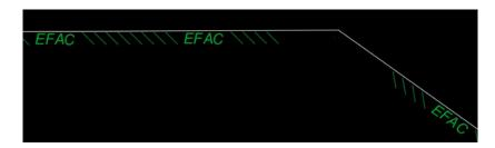
Use block RW-EAC for additional slash marks. The block can be mirrored if the slash marks need to go in the opposite direction. If there are too many slash marks for the line segment, explode the block after it is in place and delete the extra slash marks.
