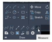
Within the Measure command, select the object to measure (the r/w line), select Block, and enter the block name (RW-FAC or RW-LAC). Select Yes when asked to Align block with object. For specify length of segment enter a value that is 2 times the drawing scale (400 for 200 scale, 200 for 100 scale, 100 for 50 scale).
