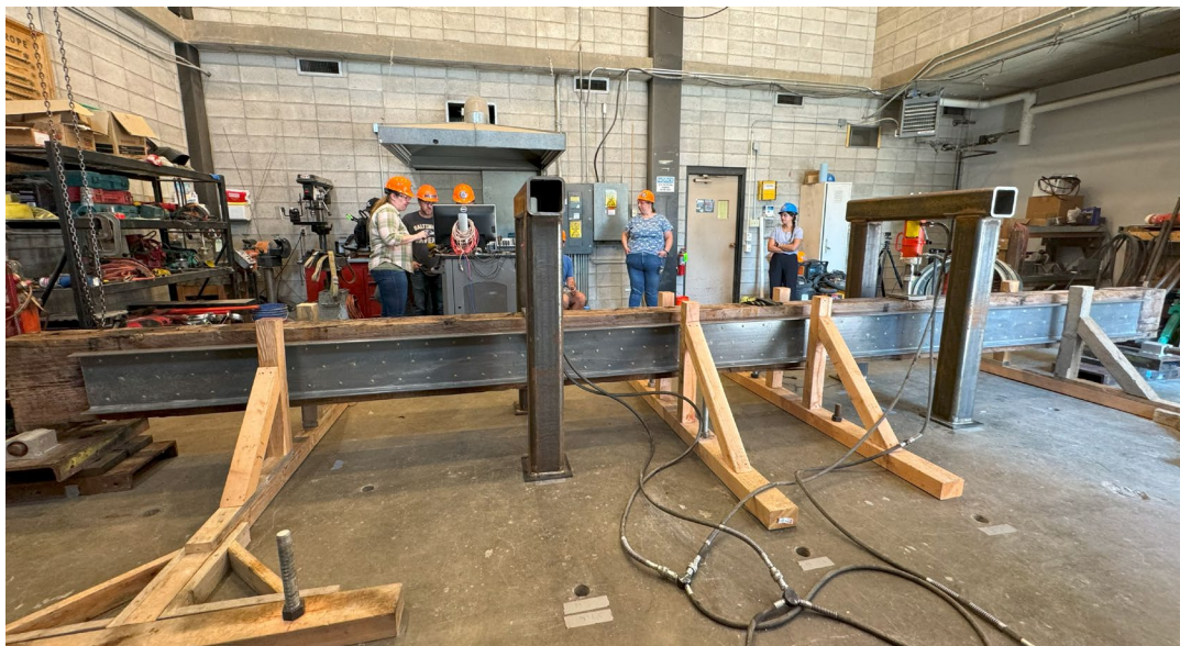
Figure 46: 8"x18" split repair beam with C-S tested in flexure setup - 8-Fl-SR(C-S)
