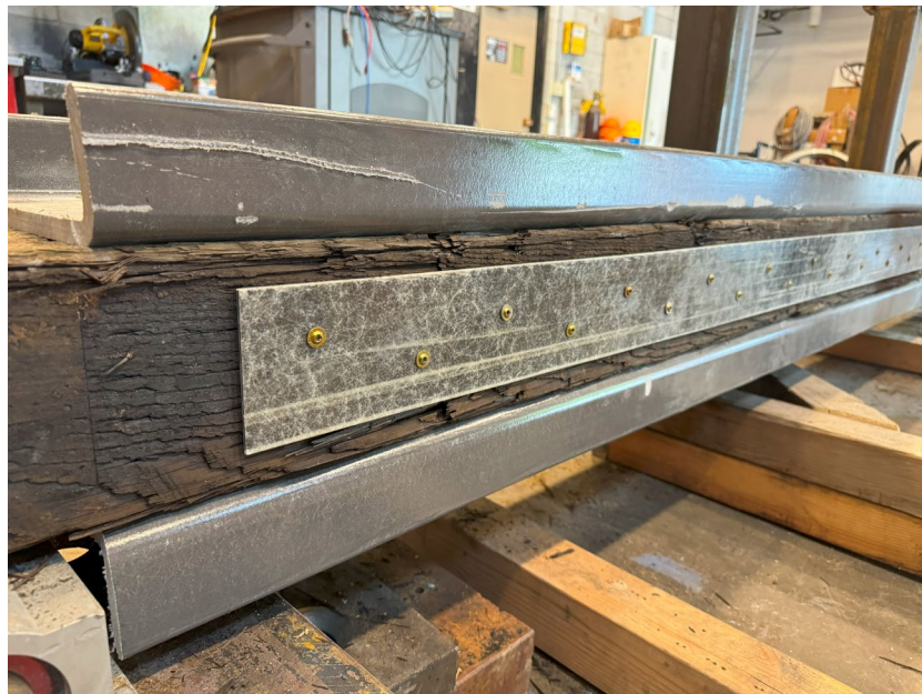
Figure 7: Example timber beam with FRP materials attached
