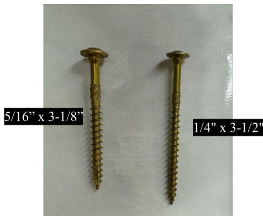
(a) RSS-GRK screws for attaching FRP to timber beams
