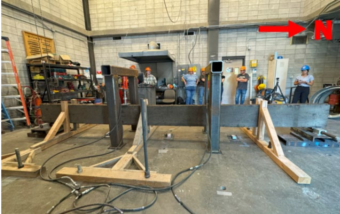
Figure 36: Flexure test setup for 19' span beam
