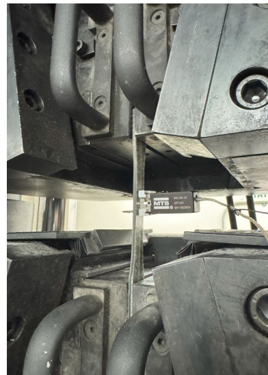
(b) Hybrid FRP strip coupon
