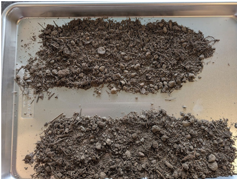
Figure 8. Soil sample on a tray after being dried in the oven.
