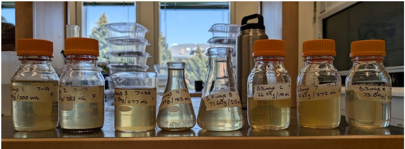
Figure 11. Soil water mixture after treatment with ferric sulfate and filtration.
