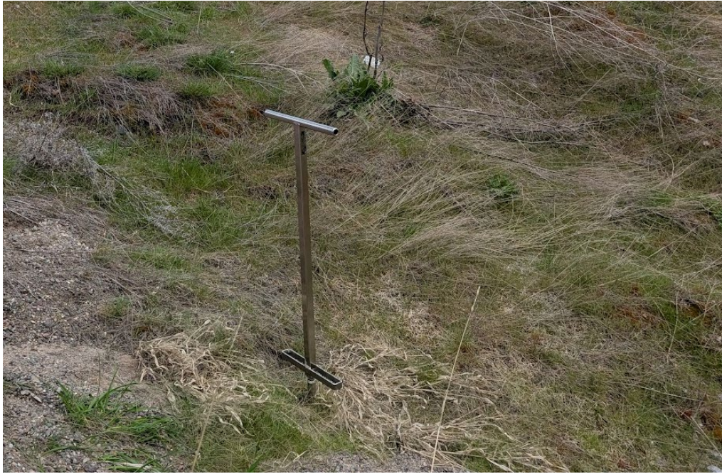
Figure 5: Soil probe in the field.
