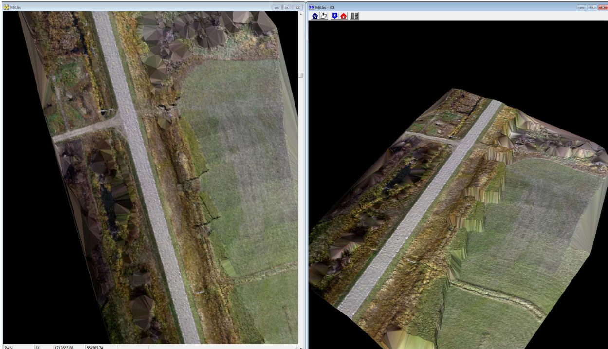
Colorized TIN showing stepping created by airframe altitude variation
