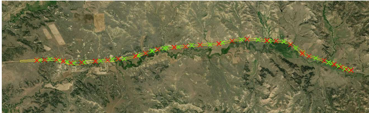
Ashland Corridor Control (X = Ground Control Point, X = Check Point)
