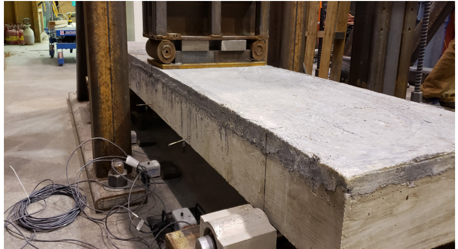
UHPC samples undergo testing to evaluate the material's potential in different applications.
