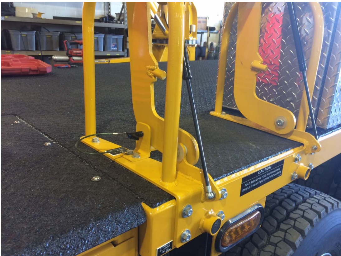
The left hand deck step must be stowed and retainer pin in place, for road travel.
