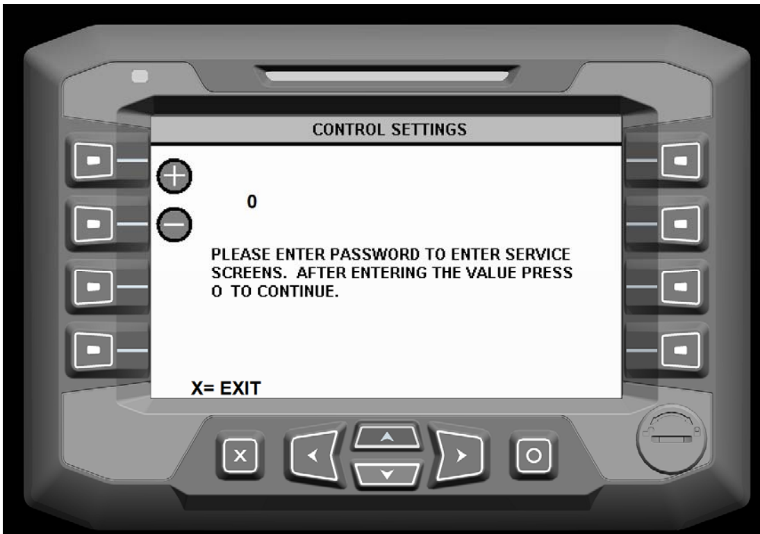
A Password Must be Entered to Gain Access to the Control Settings Screen
