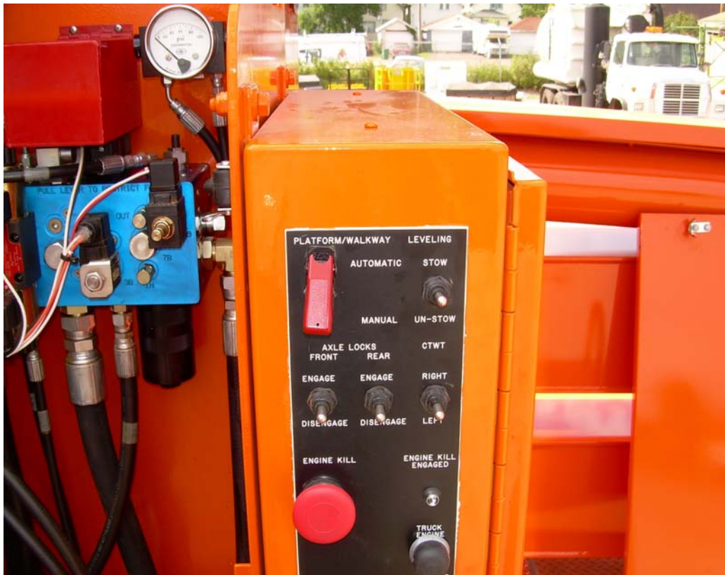
LEVEL THE PLATFORM USING THE SWITCH AT TURNTABLE 1 LED BOX
