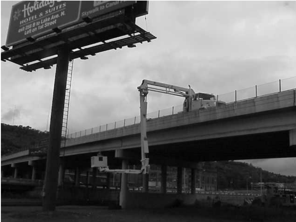
BOOMS #2 AND #3 HAVE NOW BEEN OPERATED TO "OPEN" SUFFICIENTLY TO ENABLE PLATFORM TO BE POSITIONED UNDER THE BRIDGE DECK
