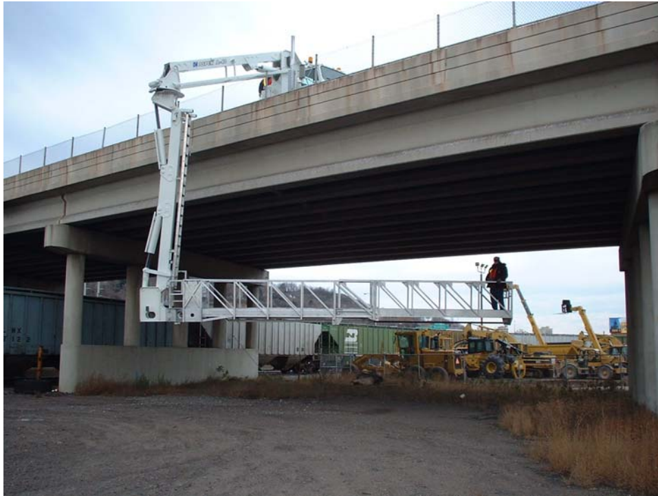
T2 BEING ROTATE CLOCKWISE TO BRING PLATFORM FORWARD
