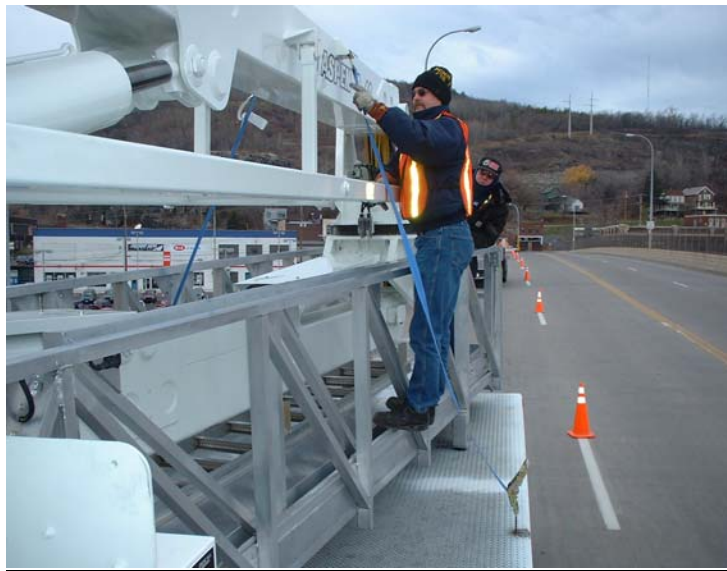
PARK UNIT AT THE BRIDGE, ENGAGE AXLE LOCKS AND RELEASE BOOM TIE DOWN DEVICE
