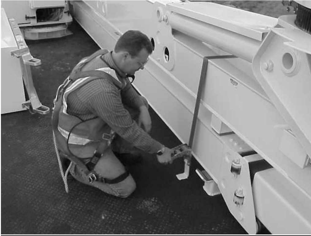
RELEASE THE BOOM TIE DOWN DEVICE
