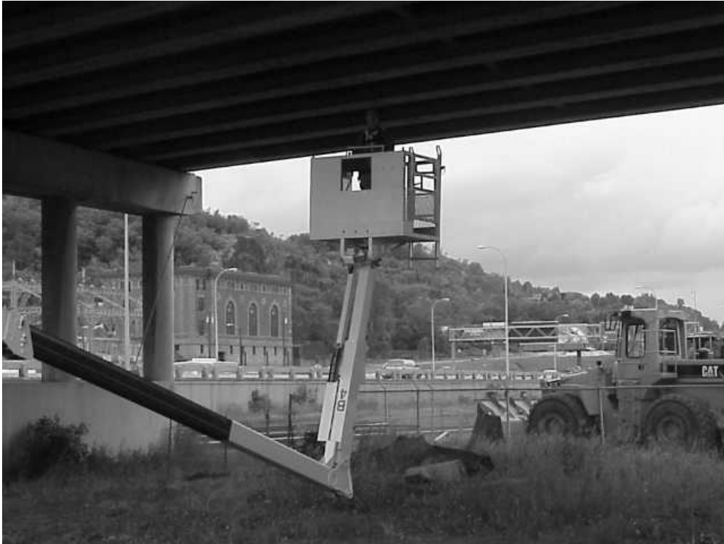
BOOM #4 MAY NOW BE TELESCOPED IN AND OUT
