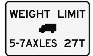
The posting on the South Fork McDonald Creek Bridge applies to SHVs; it limits the maximum gross vehicle weight of single-unit vehicles with 5, 6, or 7 axles to 27 tons.
