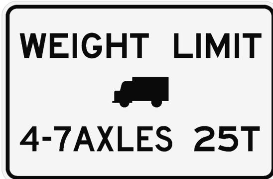
The new posting on the Skull Creek Bridge applies to SHVs; it limits the maximum gross vehicle weight of single-unit vehicles with 4, 5, 6, or 7 axles to 25 tons.
