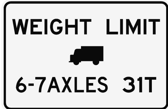
The new posting on the Red Lodge Creek Bridge applies to SHVs; it limits the maximum gross vehicle weight of single-unit vehicles with 6 or 7 axles to 31 tons.
