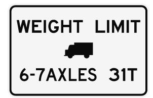
The new posting on the Butte Creek Bridge applies to SHVs; it limits the maximum gross vehicle weight of single-unit vehicles with 6 or 7 axles to 31 tons.
