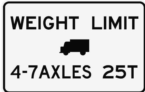
The new posting on the Coffee Creek Bridge applies to SHVs; it limits the maximum gross vehicle weight of single-unit vehicles with 4, 5, 6, or 7 axles to 25 tons.
