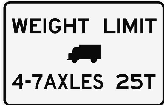
The new posting on the N Fork First Hay Creek Bridge applies to SHVs; it limits the maximum gross vehicle weight of single-unit vehicles with 4, 5, 6, or 7 axles to 25 tons.
