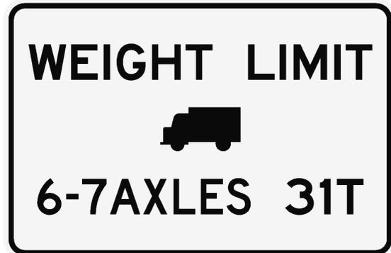
The new posting on the Redwater River Bridge applies to SHVs; it limits the maximum gross vehicle weight of single-unit vehicles with 6 or 7 axles to 31 tons.
