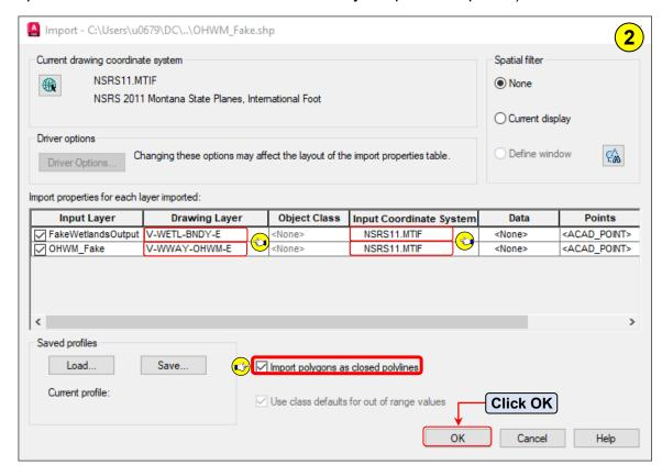
Note: For the "Input Coordinate System" column > select the cell > select browse button > from the coordinate system dialog box > type NSRS11.MTIF (Or appropriate coordinate system matching the survey file if not NSRS11.MTIF) in the search box > select the coordinate system > click Select. Repeat for all Layers.
