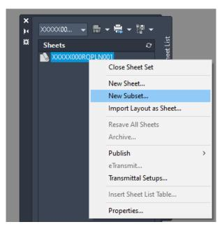
Inside the Subset Properties dialog box rename the subset to "RIGHT OF WAY PLAN", this will allow the SSM to change the name of every sheet (ROTTL, ROOWN, ROPLN) in the bottom right corner of the page. Verify the sheet location is in the Autodesk Docs RO Folder, then select OK.
