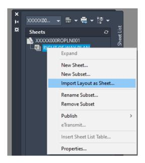
Inside the Import Layouts as Sheets dialog box, select 'Browse for Drawings...'. Select the ROTTL sheet as well as any other created sheets (ROOWN, ROPLN). Click 'Open'. Select the desired layouts by clicking inside the check box in front of the drawing name(s). Verify that any unwanted layouts (e.g. MDT-TMP) are unselected before clicking 'Import Checked'. The selected layouts will be added to the RIGHT OF WAY PLAN subset.
