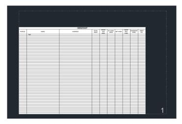
Select the sheet and move its insertion to the top left of the viewport using the move command (M).
