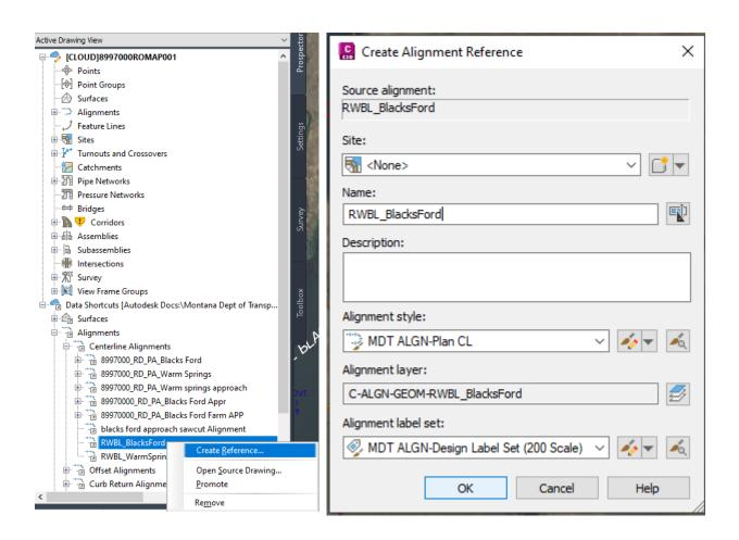
In the 'Create Alignment Reference' pop-up window, verify the Alignment style is 'MDT ALGN-Plan CL' and the Alignment label set is 'MDT ALGN-Design Label Set (200 Scale)' and select 'OK'.
