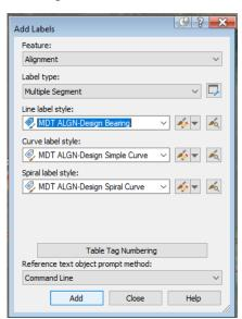
Select 'Add'. When prompted, select the alignment on screen to apply the labels to the alignment in model space.
