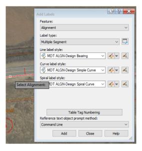
These labels can be moved using by selecting the label and grabbing the blue square grip to move in any direction or the blue diamond grip to move along the alignment.
