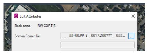
For Lines containing elevations, the command OSNAPZ system setting will disregard the vertical distance between two points and place the line connecting the two points on a zero-elevation plane. OSNAPZ Has two settings, 0 and 1.0 is default and keeps the vertical distance and 1 disregards the vertical distance. For R/W Plan Production, Section Tie Distances are 2D grid distances.
