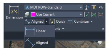
The default layer is set to Use Current, however a layer can be set from the dropdown for all dimensions created. Verify dimensions are placed on the correct layer.
