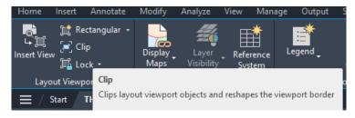
Select the viewport, on the command line select Polygonal and draw a polyline around the clip area and select Close. You cannot snap exactly to the intersection of the match line and the sheet border; the polyline location will be approximate. The polyline can be edited by clicking on the vertex points to show the desired view. There may be multiple objects on top of each other. Toggle on Selection Cycling to make it easier to pick the viewport.
