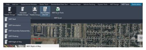
Blocks with associated attributes will prompt during placement of the block to populate the fields of the block. When placing blocks with associated attributes, do not copy blocks, use the R/W Block Palette in the Tool Palettes only.
