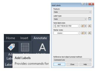
In the Add Labels dialog window, set the feature to note, label type to Note and in the Note label style, select the style accordingly. Verify the marker style is set to None. Select Add and snap to the existing R/W line. Move and rotate the label by selecting it and grabbing the square grip.
