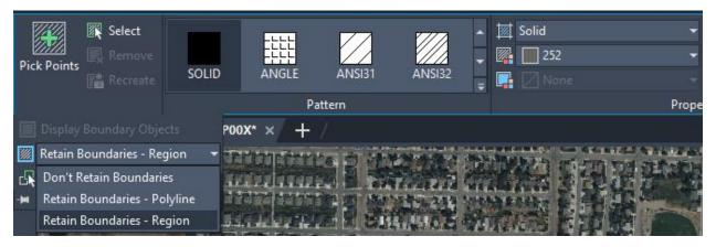
If an message come up saying "a closed boundary could not be determined" create a boundary to make a closed shape. If the area is along strait lines, trace the shape with a polyline and close the polyline. If the area is along a curve, use NCOPY to copy lines from reference files in place, unload the reference files and use the Modify tools to create a closed shape. After the closed boundary has been created use the directions above to create a hatch (fill area).
