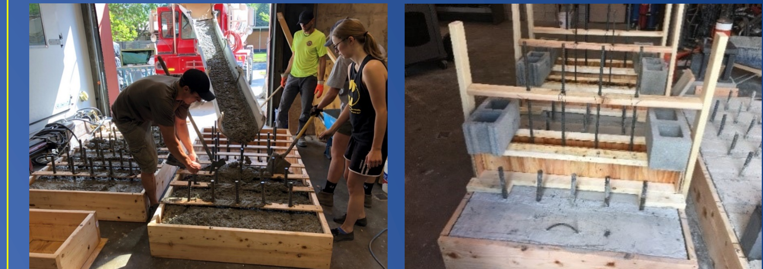
Test Specimens During and After Construction
