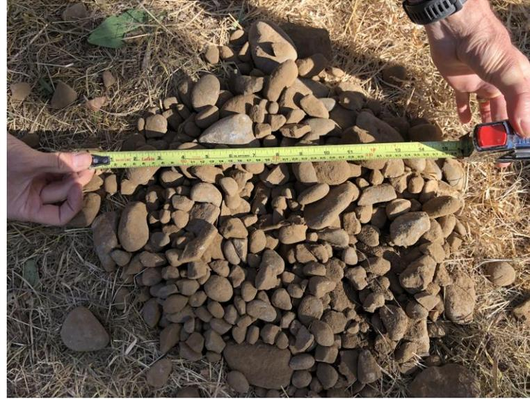
Large Gravel Particles cannot be sampled using SPT and N value will be affected by Gravel. If SPT is the only option measure N value for **every inch penetration.**
