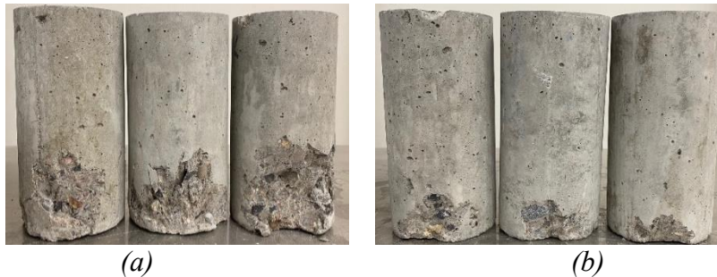
Figure 79. Two proposed Concrete Mixtures after 28-day Strength Test
