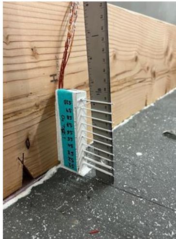
Figure 110. Temperature sensor for monitoring thermal behavior of snow
