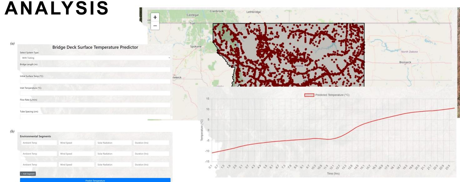
Developed an interactive web-based portal that allows users to estimate bridge surface temperatures under various design and climate conditions
