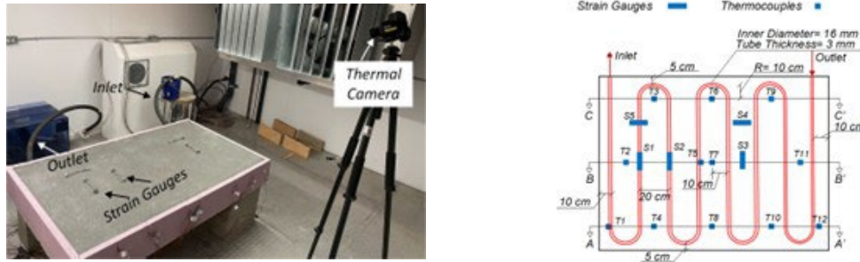
Figure 1. Bridge deck model (left) and instrumentation schematic (right), with thermocouple and strain gauge locations shown
