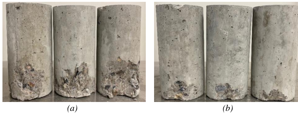
Figure 5. Two proposed Concrete Mixtures after 28-day Strength Test
