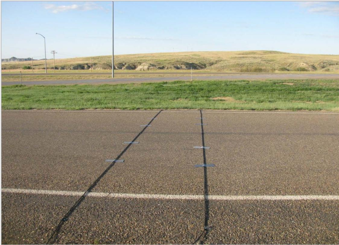
**Figure 3-3: Pneumatic Tube Setup**
