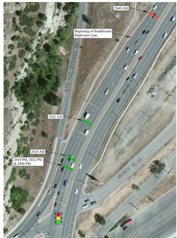
Figure 9 Southbound-Through 95th Percentile Queue Length Locations at 6th Ave/Main St
