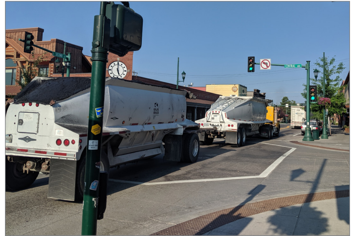
Trucks with long trailers frequently travel through Downtown Whitefish. Limited queue storage space can cause vehicles to block intersections and impede traffic flow.
