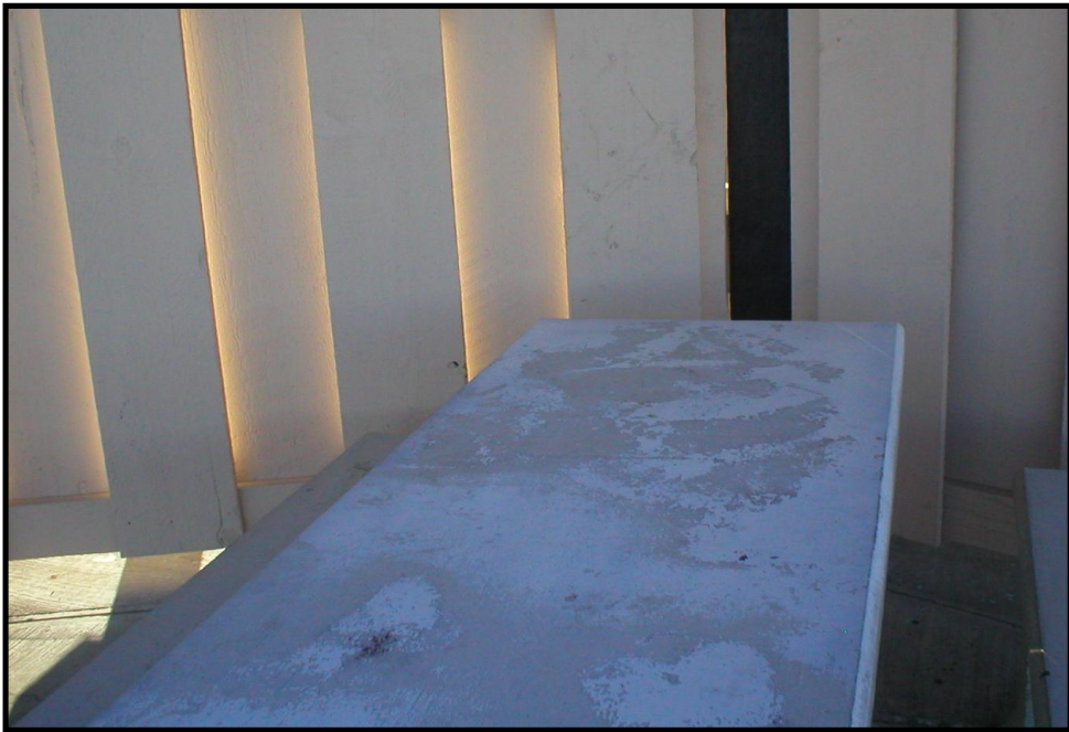
Photo 16. Chipping paint on picnic table at Hathaway EB site.
