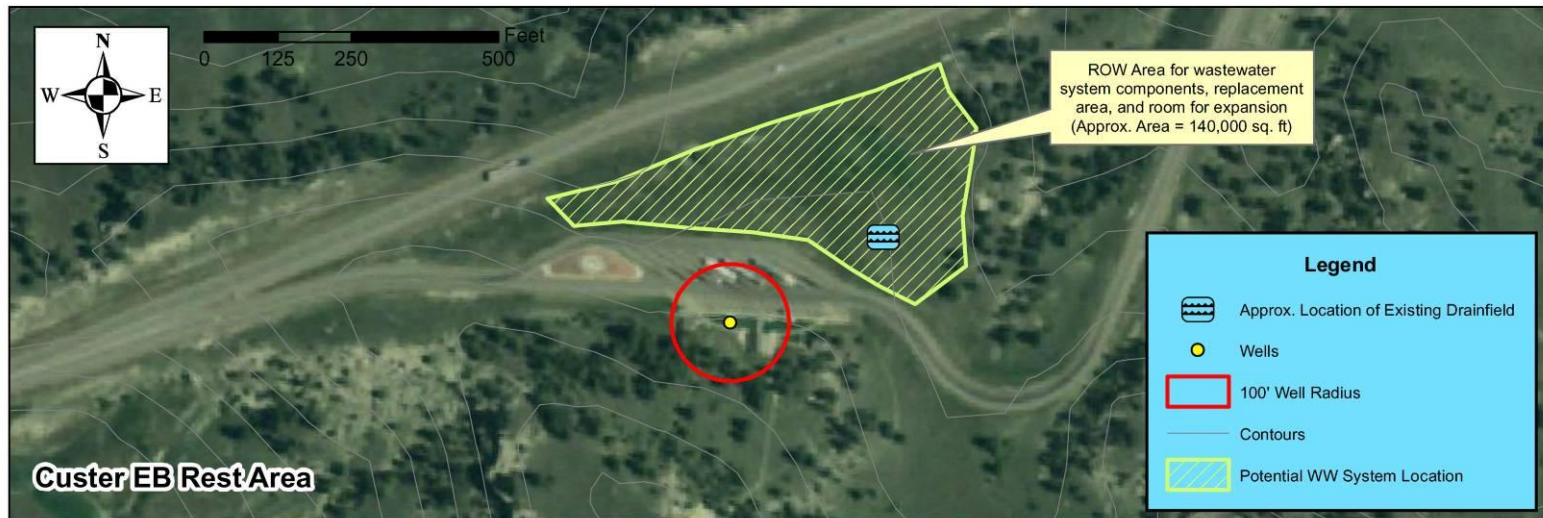
Figure 3-19 Custer Conceptual Wastewater Treatment System
