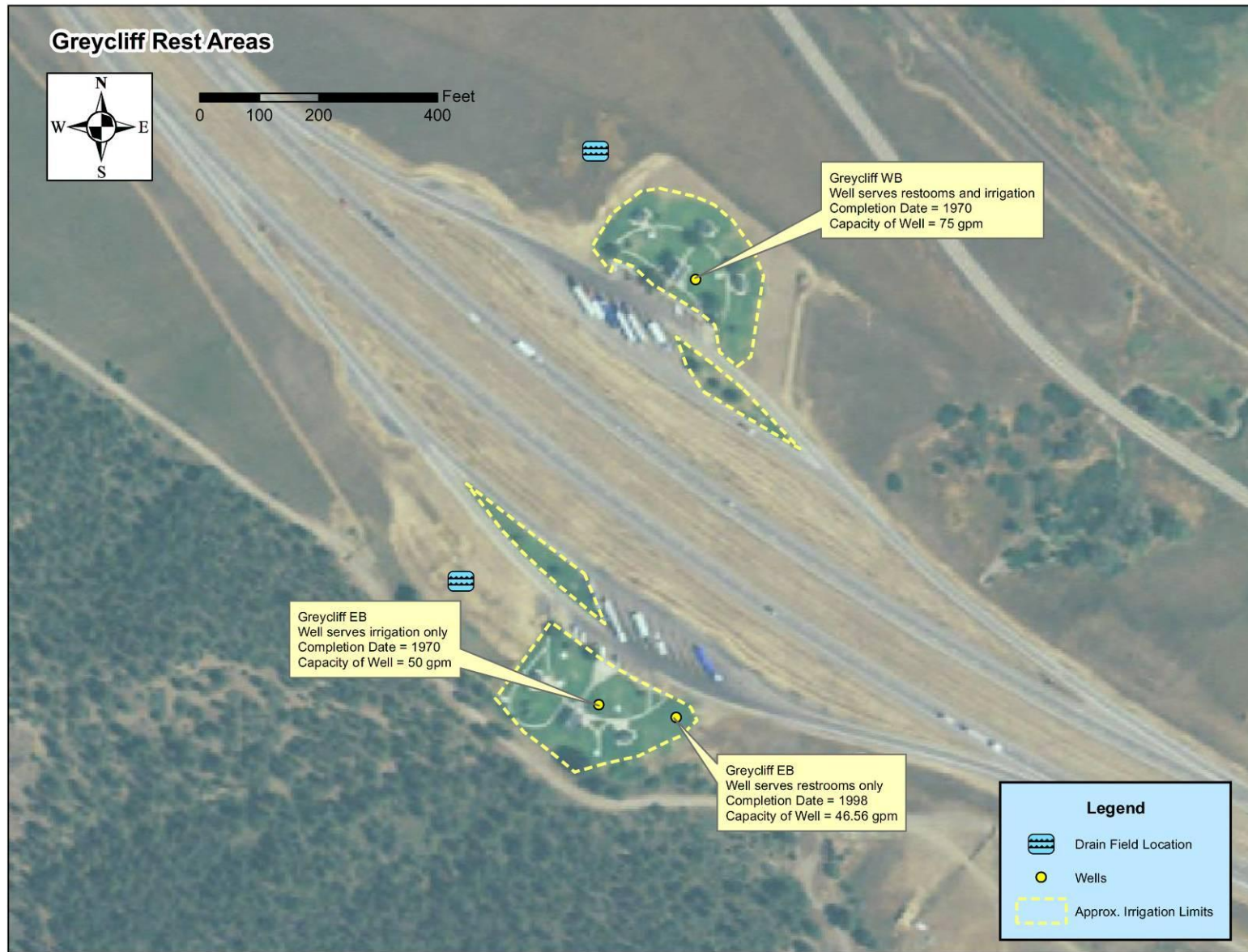
Figure 2-6 Greycliff Water and Sewer Location Map
