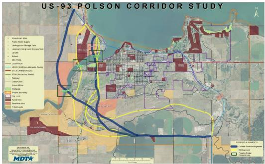
Community input, coupled with direction from the TOC, led to slight modifications of the five selected alignments to minimize residential impacts near Ponderrilla Hills. Since the original EIS alignments 2 and 3 are relatively close to the Quantm generated alignments of the southern bridge crossing and the northern bridge crossing, a hybrid was developed between the southern bridge crossing alignment and EIS Alignment 3.
